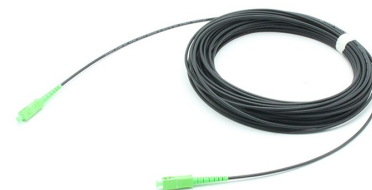
3.0mm LSZH SCAPC-SCAPC G657A2 Round FTTH Drop cable patch cord
