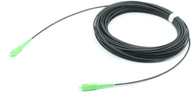
3.0mm LSZH SCAPC-SCAPC G657A2 Round FTTH Drop cable patch cord
