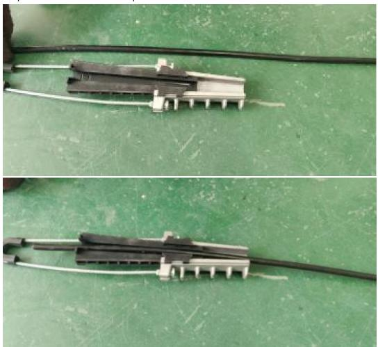
Step 3: Adjust the position of the wire and pull the core back into the aluminum body.
