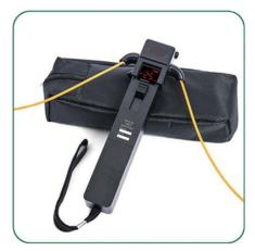
The Live Fiber Identifier allows you to detect traffic and measure signals anywhere On single mode fibers without having to disconnect them. It also lets you check for signal presence before rerouting or maintenance, perform continuity tests and verify cable labeling. Based on non-destructive macro bending technology, it doesn't disrupt traffic, damage or overstress the fiber, enabling efficient, accurate and reliable data acquisition
