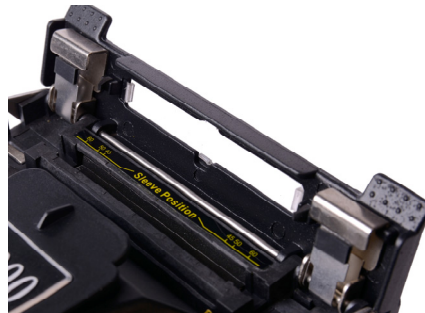
Automatic inductive heater Not heating without fiber
