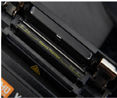
Inductive automatic heater Not heating without fiber
