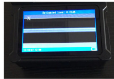
Splicing after dropping from 76cm
