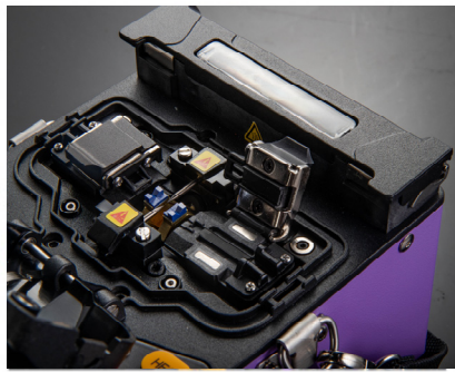
Precise V groove design Stable splicing performance
