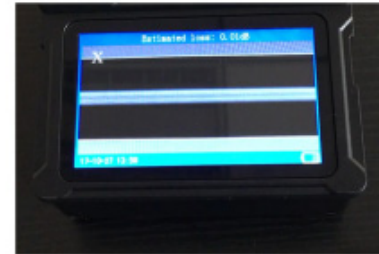
Splicing after dropping from 76cm
