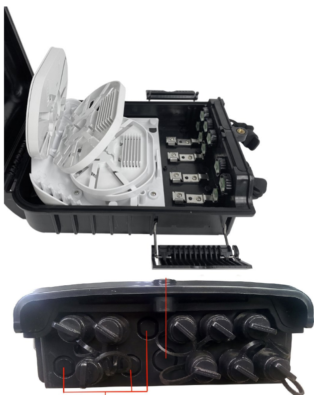
Reserved hole for waterproof Pre-connectorized SCAPC adapter
