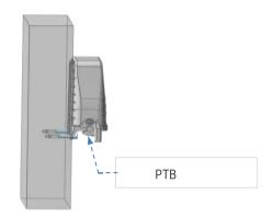
Drill 2 holes into the wall, place the expansion bolt  $\Phi$ 7.5\*40, place the box to match up the holes and use bolt to fasten
