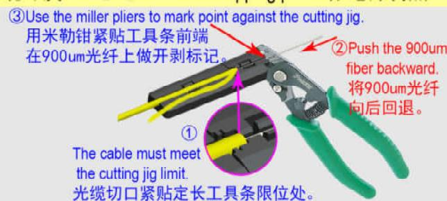
③ Use the miller pliers to mark point against the cutting jig.
