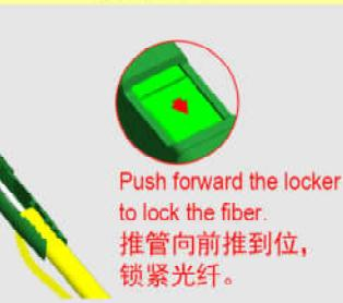
Push forward the locker to lock the fiber.
