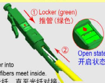
Insert the fiber into connector, till fibers meet inside.
