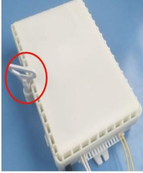
2. Strip the cable, remove the outer and inner sheath, lose tube, clean and remove the filling paste in the cable, leave 0.6~1.2m bare fiber and 30-50mm steel core, pass the cable into the box through the inlet, fix it with hose clamp, fasten the re-enforced core.
