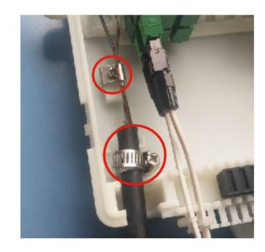
4. Fix the steel pipe PLC in its special slot on the back of the flip board, coil the output pigtails and connect them to the adaptors; lead the incoming pigtail into the splicing slot from the notches on both side of the flip board, splice it with the incoming fiber.
